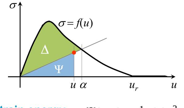
**strain energy**  $\Psi(u, \alpha) = \frac{1}{2}g(\alpha)u^2$ **dissipation**  $\Delta(\alpha) = \int_{0}^{\alpha} f(s)ds - \frac{1}{2}g(\alpha)\alpha^2$
