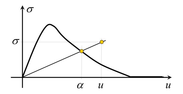
but  $\sigma = f(u)$  is again the border of the elastic zone, and  $\alpha$  is again the intersection of the loading curve  $\sigma = f(u)$  with the straight line joining the point  $(\sigma, u)$  and the origin with the addition of the viscous term, the power equation becomes  $(\sigma - g(\alpha)u)\dot{u} + \frac{1}{2}g'(\alpha)(\alpha^2 - u^2)\dot{\alpha} - \frac{1}{2}h(\alpha)\dot{\alpha}^2 = 0$
