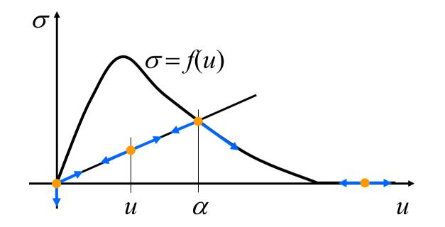
the desired response has been obtained by a proper choice of the potentials, assuming energy conservation and dissipation principle
