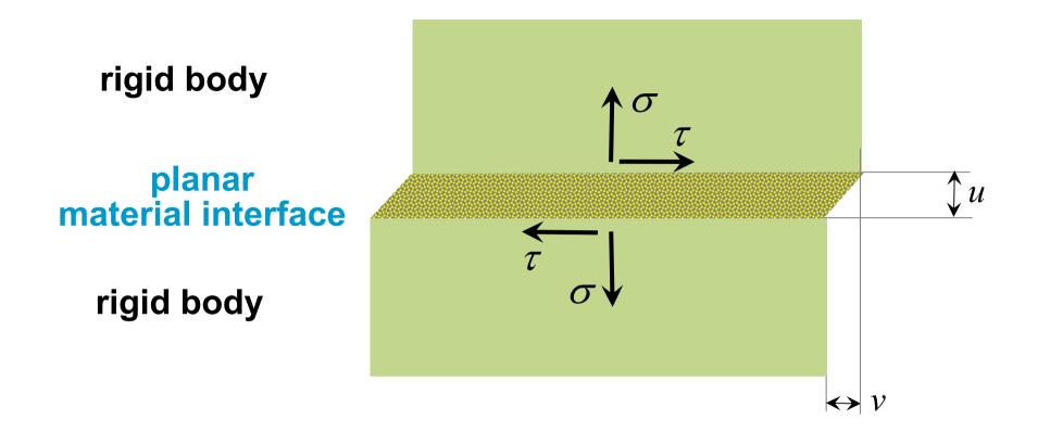
u, v: normal and tangential relative displacements  $\sigma, \tau$ : normal and tangential forces
